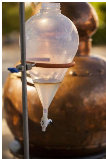
Figure 1.4 illustrates the separation of the hydrosol and the essential oil in the collection vessel once the distillation process is complete.
